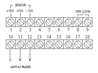
Pin 1 : +10V supply for turbine flow sensor Pin 2 : Positive input for signal from sensor Pin 3 : Negative input for signal from sensor Pin 8&9: Configuration Lock (Open to lock)
